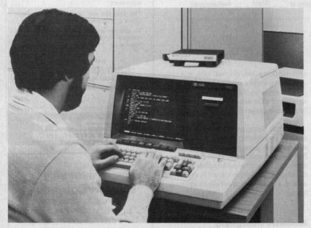
The basic Hewlett-Packard Model 64005S emulation terminal system includes a development station with a cartridge tape drive and emulation hardware/software for the selected microprocessor. Directed syntax through eight soft keys works to eliminate syntax errors.
