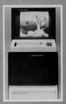
A compact entry-level system, Comtal's Vision One/10 stand-alone digital image processing system has many of the state-of-the-art capabilities of the company's more powerful Vision One/20 system.
